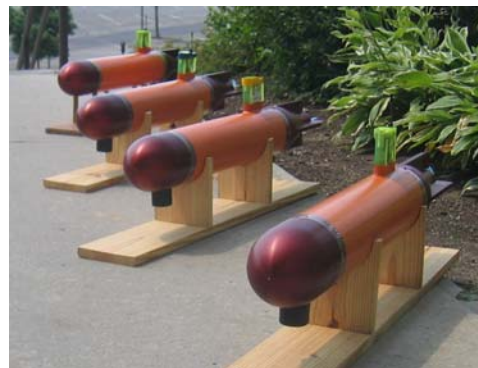
Several Virginia Tech 475 autonomous underwater vehicles (The outside diameter of these AUVs is 4.75 inches.)
