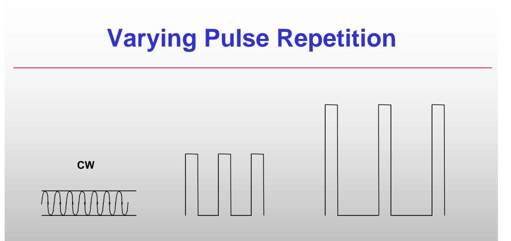
All three signals could produce the same result on a CISPR receiver using the QP detector
