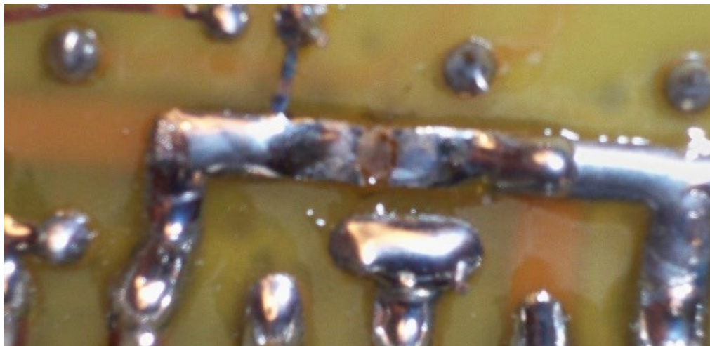
Figure 17: Blown PCB Trace
