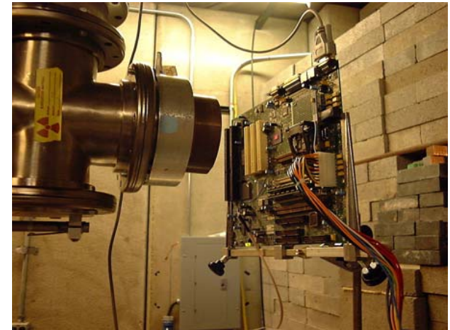
Heavy ion SEE test setup (SOURCE: JPL)
