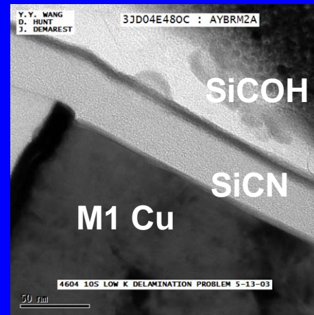
TEM of Delaminated Interface
