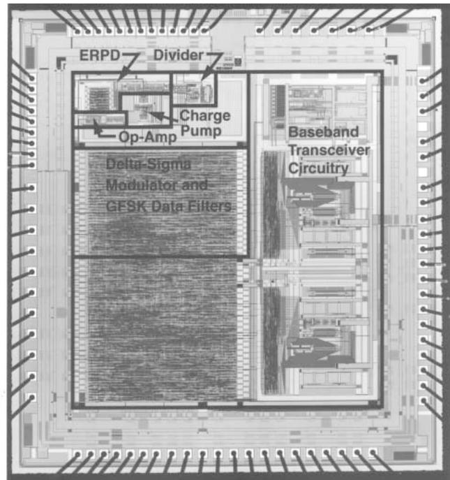
**Figure 12.3.8: Prototype SWAP transceiver chip micrograph.**
