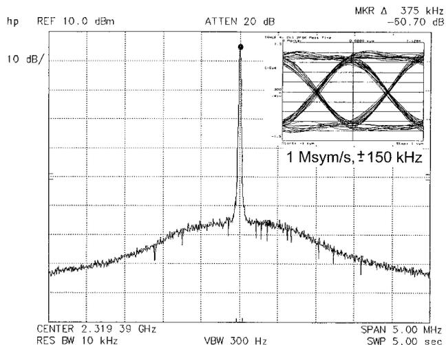
Figure 12.3.6: Unmodulated carrier spectrum (receive mode, 2319MHz) and modulated FSK eye diagram (transmit mode, 2430MHz).
