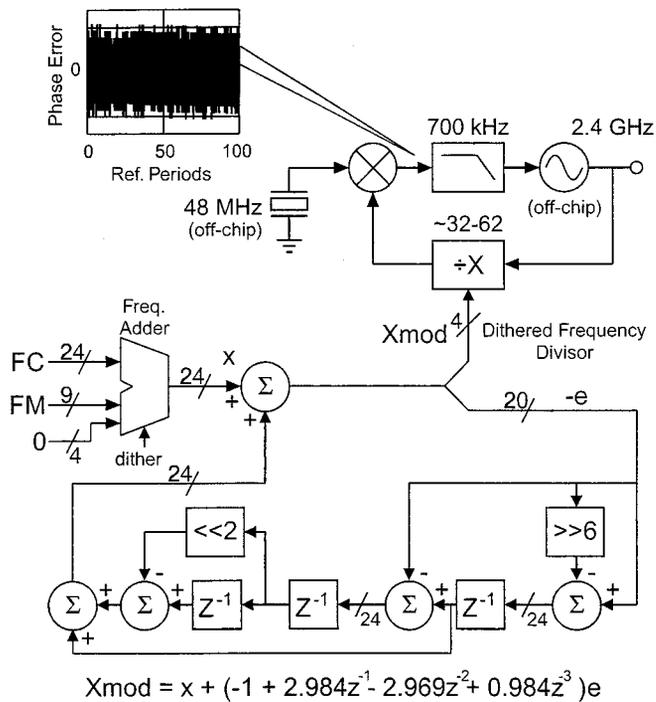
Figure 12.3.1: Block diagram of the wideband FN synthesizer PLL.
