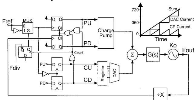
Figure 12.3.3: The extended-range phase detector concept.
