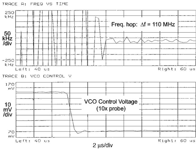
**Figure 12.3.7: Frequency hop settling vs. time.**
