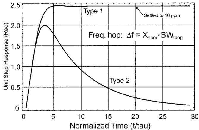
Figure 12.3.2: Ideal phase error transients of type-1 and type-2 PLLs.
