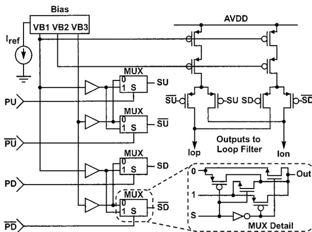
Figure 12.3.4: Charge pump schematic.
