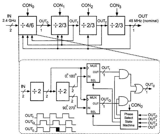
Figure 12.3.5: The high speed multi-modulus divider.
