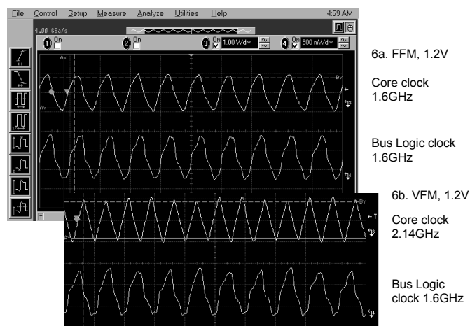
Figure 16.2.6: FFM/VFM core/bus clock oscilloscope traces.
