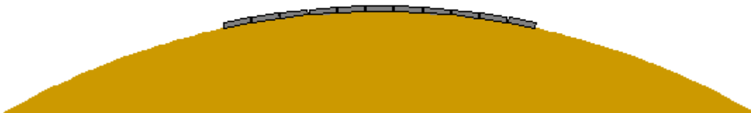
Figure 8 – Side view of the 1.41mm x 1.41mm cells bending around a 4” diameter object. As expected, with smaller cells, the curve of the object is followed more closely.
