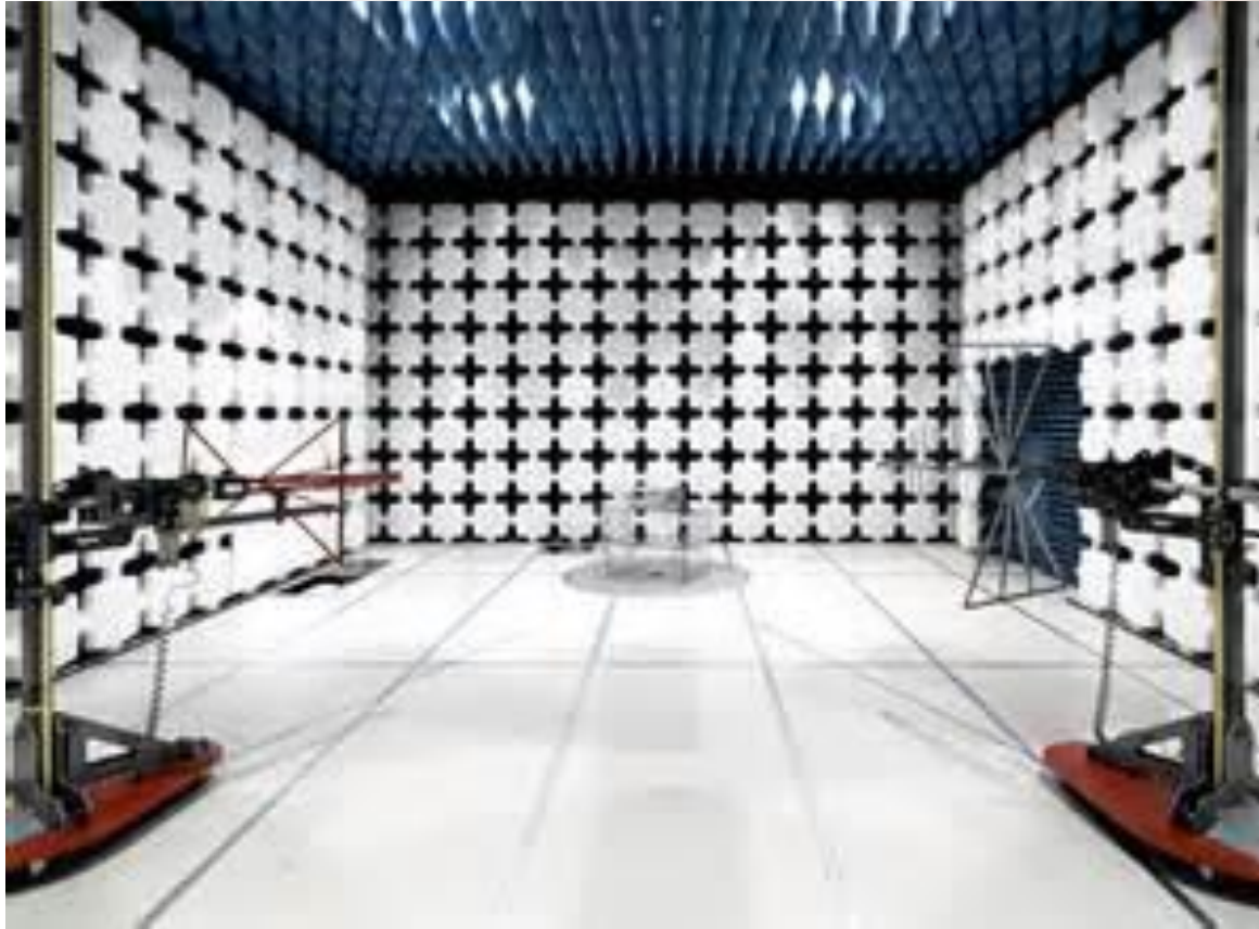
Semi-Anechoic 10m Chamber
