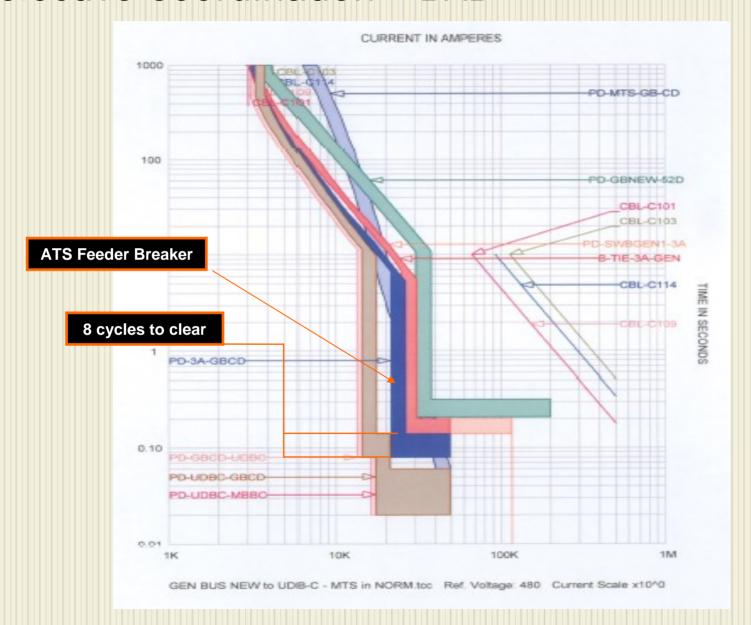
In this case, since it takes 8 cycles for the upstream breaker to clear the fault, a 3 cycle rated transfer switch is inadequate.
