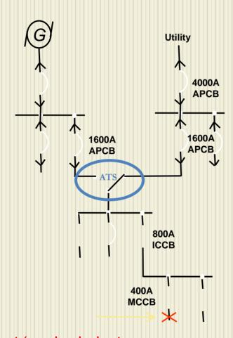
MCCB's (Molded Case Circuit Breaker) Instantaneous or Current Limiting Devices.
