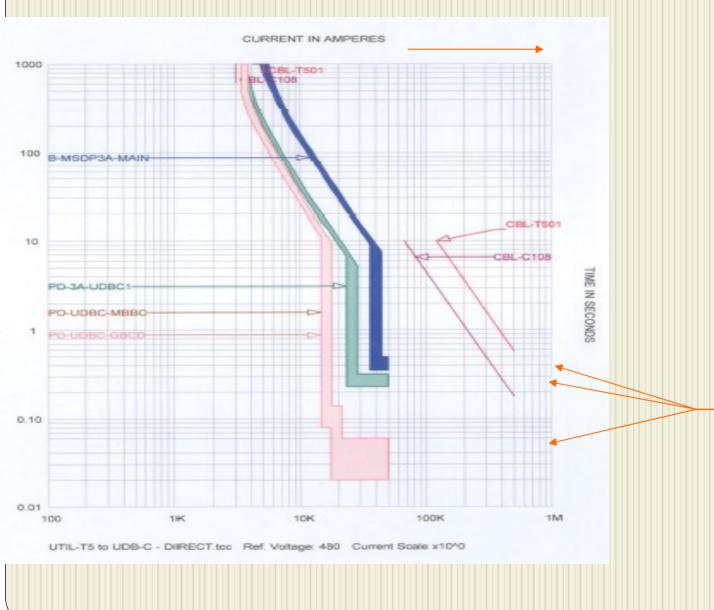
No overlapping fault current of individual devices.
