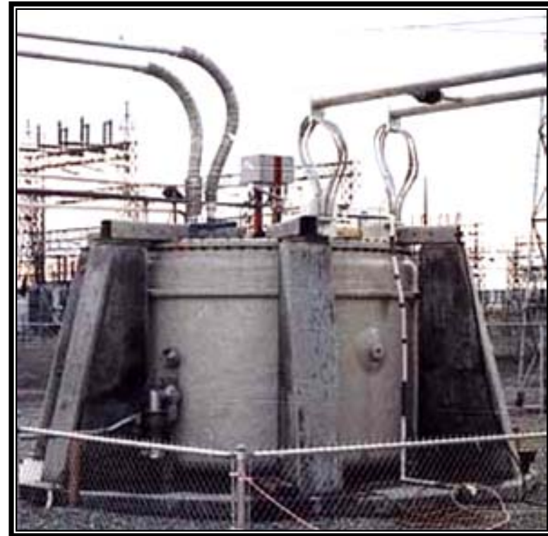
10 MW – 3 Sec. Coil Tested For Transmission Stability
