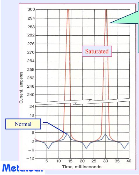
Transformers easily *Saturate* with even minor levels of GIC
