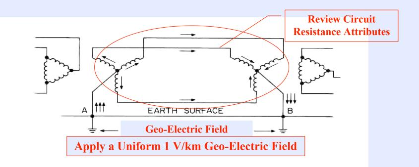
A Simple 100 km Transmission Line and Transformer Connections to Ground *Illustrates GIC Flow Circuit Principles for More Complex Network Topologies*
