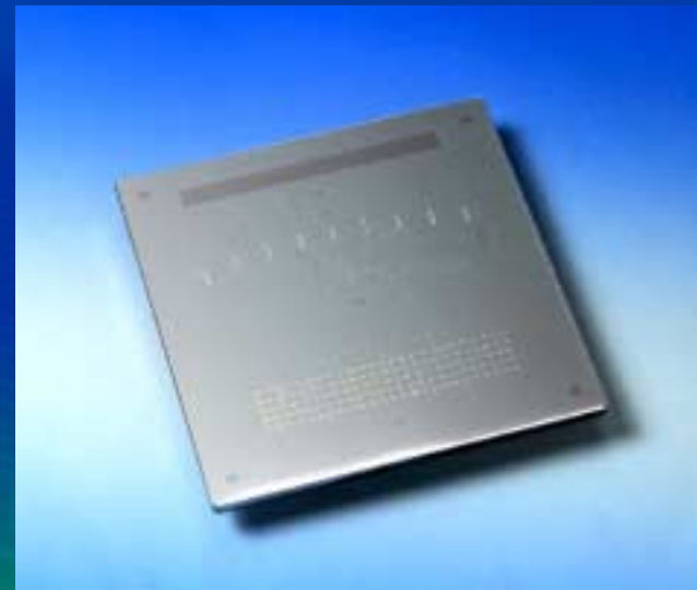
World's First 6-inch EUV ETS Mask
