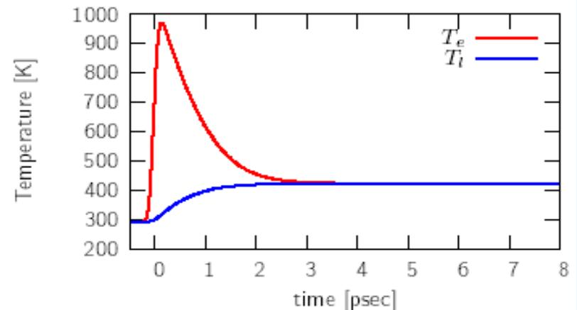
⇒ perform Langevin dynamics simulation with  $T_e$  as temperature of the heat bath
