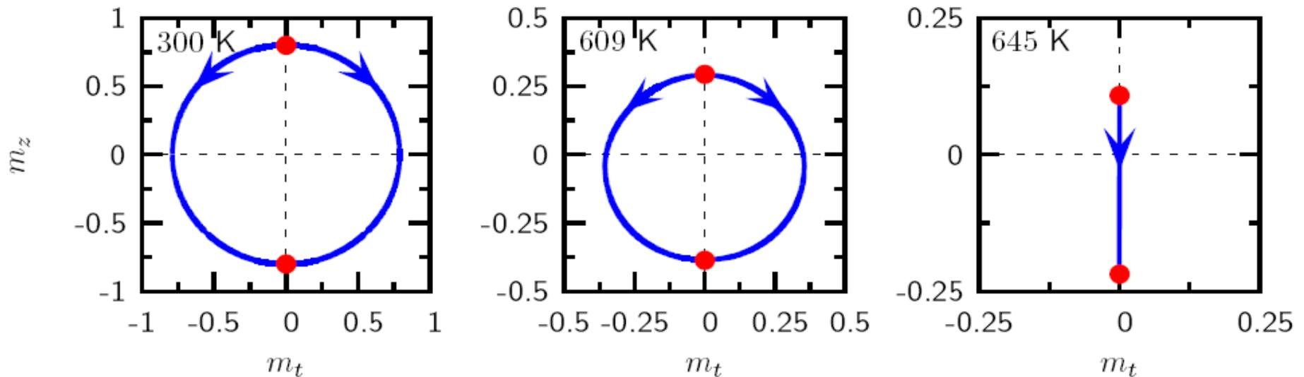
New reversal mechanism via a strongly non-uniform (demagnetised) state.
