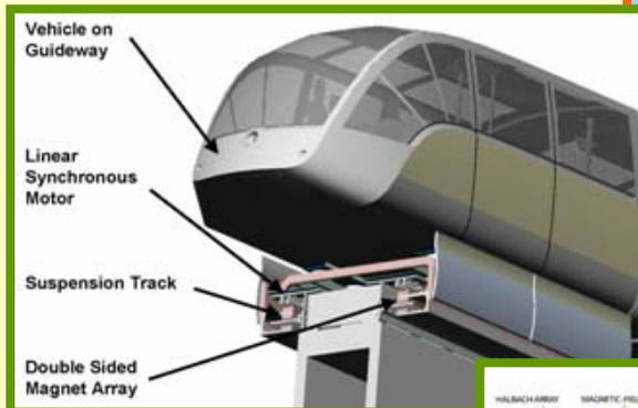
Efficient and fail-safe *Inductrack* maglev train
