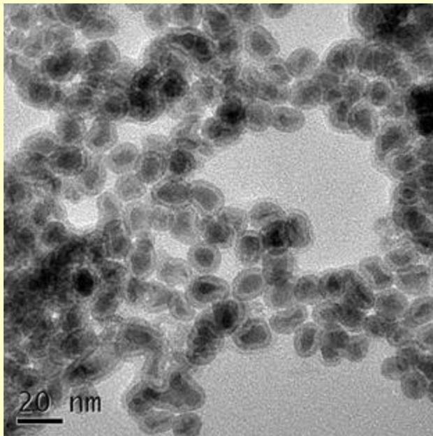
Spherical aggregates of Fe nanoparticles and surface passivation layer
