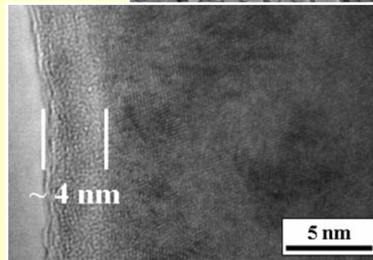
✧ The Northeastern University group (**Prof. V.G. Harris**) used a modified polyol reaction method to produce **Fe-Co ( $\approx$  Fe<sub>50</sub>Co<sub>50</sub>) particles 20 - 25 nm with  $M_s \approx 200$  emu/g.**
