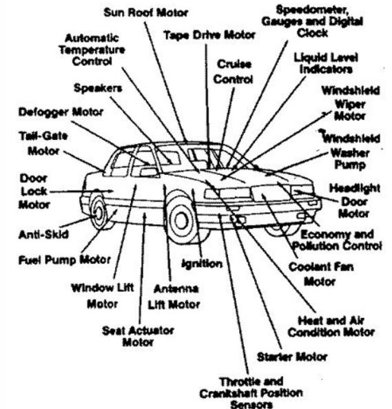
✧ In a modern car, magnets are used in more than 30 places.
