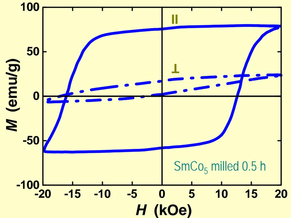
● Single crystal  $\text{Sm}_2(\text{Co,Fe})_{17}$  and  $\text{SmCo}_5$  nanoparticles can be produced by HEBM with high coercivity.
