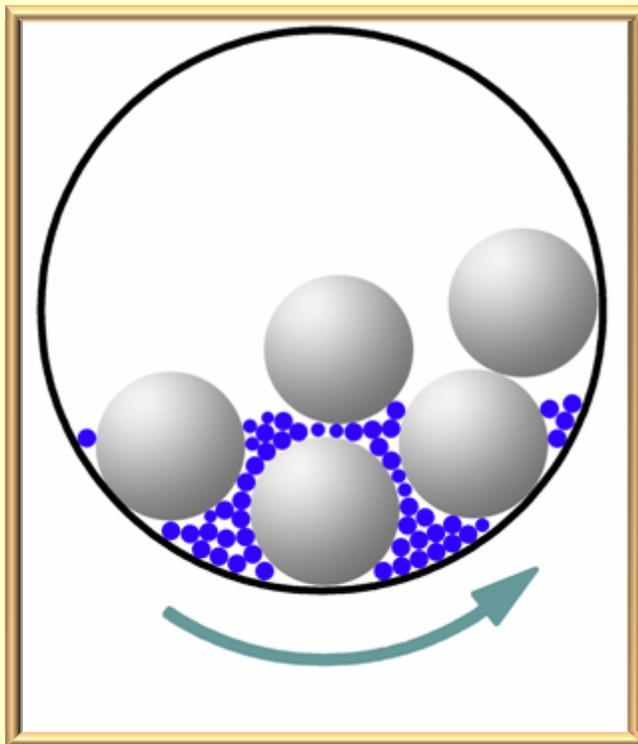
*Low-energy milling in heptane with small amount oleic acid added*
