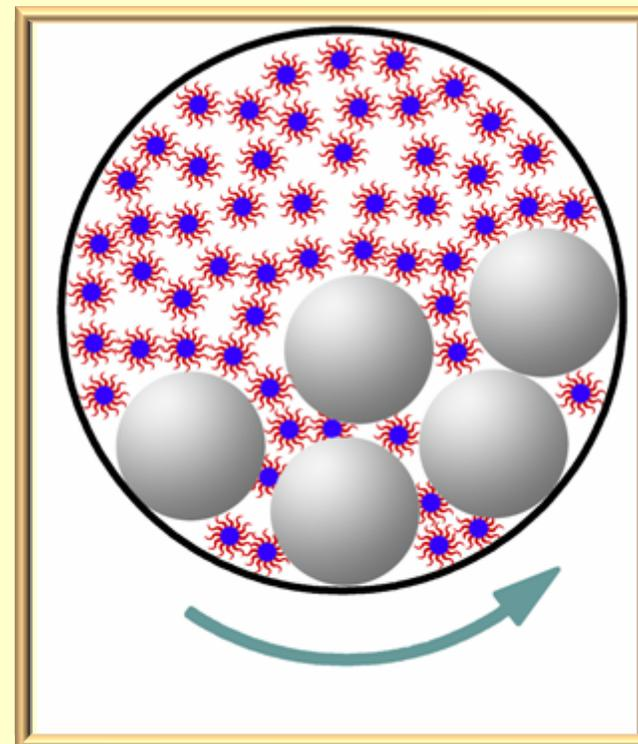
✧ Technique can be easily scaled up and it can yield **anisotropic powder**.
