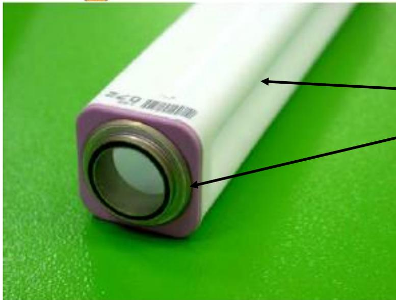
Beta alumina ceramic tube with
