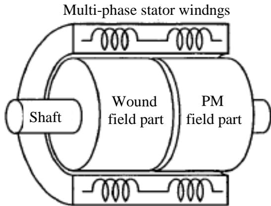
Schematic of HPM generator cross-section
