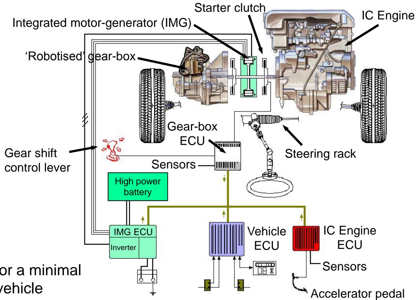
Example schematic for a minimal hybrid-electric vehicle
