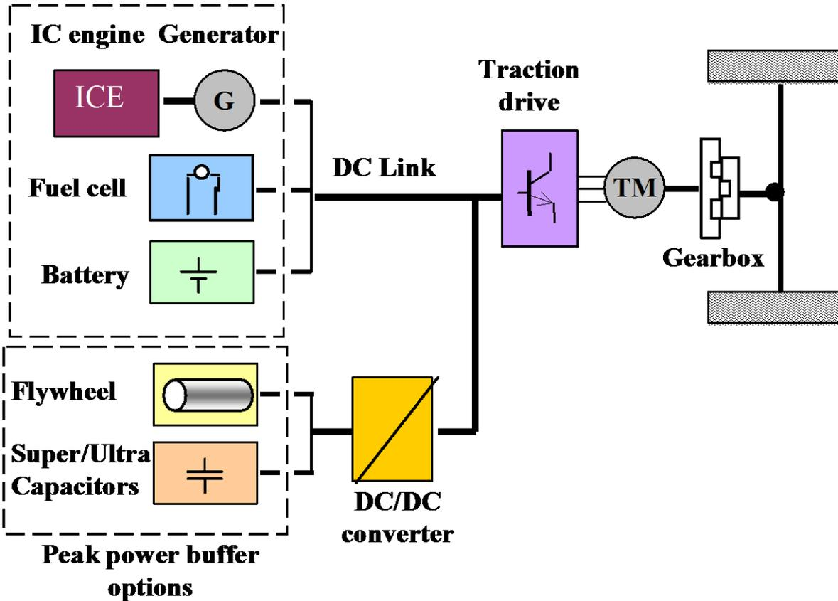
Series; dc-dc converter interfaces peak power buffer to dc-link
