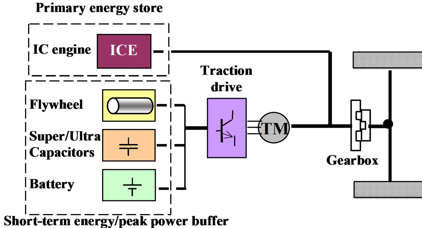
Parallel; electrical system facilitates power buffer
