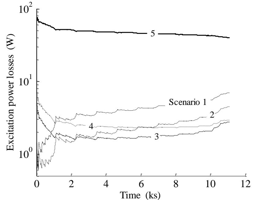
Wound field power loss during driving cycle and over battery SoC variation
