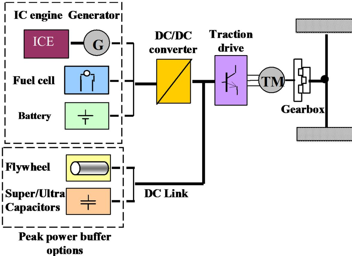
Series; dc-dc converter interfaces energy source to dc-link
