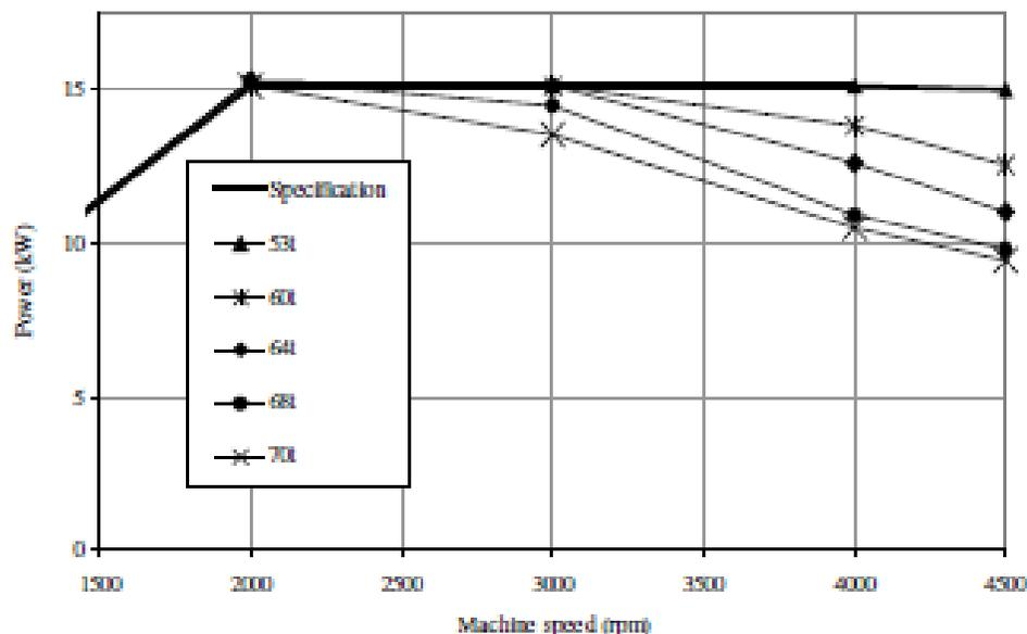
Power versus speed capability as a function of turns per stator pole
