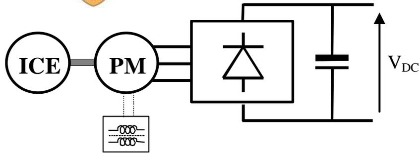
ICE/HPM machine and passive (full-bridge diode) rectification stage
