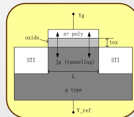
**E.G. The tunnel process cannot be expressed as a current-charge-voltage expression as Spice requires. Instead use state variables to implement tunneling correctly.**
