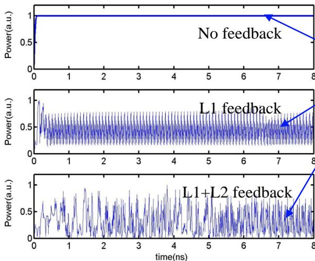
Output power degradation due to single and double lens feedback
