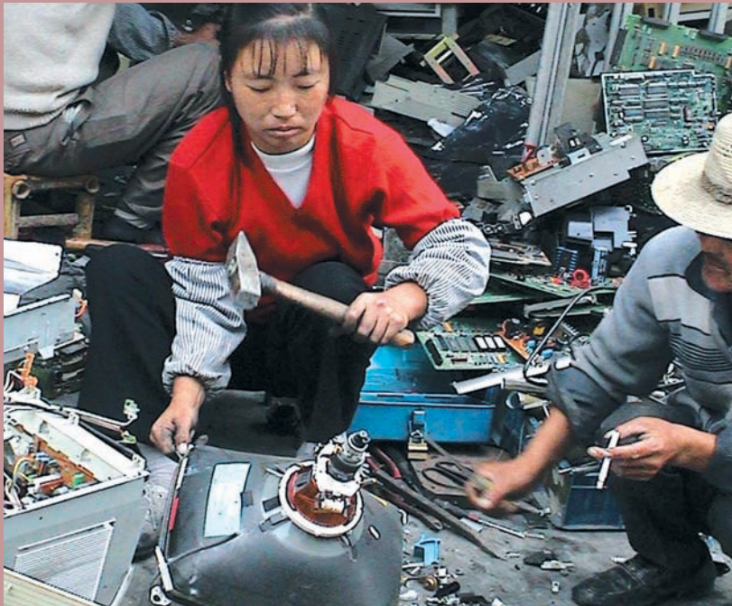
Figure 4: Woman about to smash a cathode ray tube from a computer monitor in order to remove the copper laden yoke at the end of the funnel. The glass is laden with lead but the biggest hazard from this is the inhalation of the highly toxic phosphor dust coating inside. Monitor glass is later dumped in irrigation canals and along the river where it leaches lead into groundwater. The groundwater in Guiyu is completely contaminated to the point where fresh water is trucked in constantly for drinking purposes. Guiyu, China. © Basel Action Network 2006
