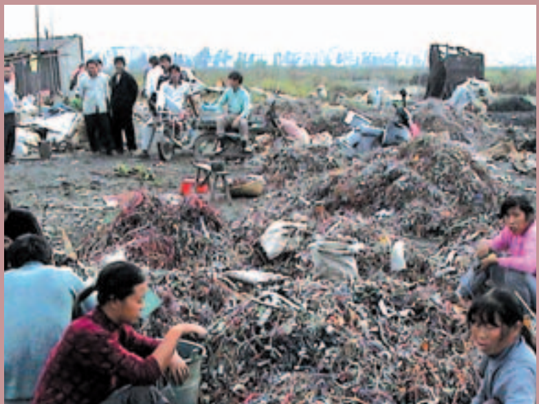
Figure 3: Women picking through wires torn out of computers. The wires are sorted by day and burned by night in this village. The families live right in the burnyards. Cancer causing polycyclic aromatic hydrocarbons and dioxins will result from burning wires made from PVC and brominated flame retardants. Guiyu, China. © Basel Action Network 2006
