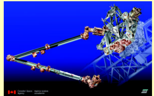
The Space Station Remote Manipulator System -- part of Canada's contribution to the International Space Station. Courtesy of Canadian Space Agency and Spar Aerospace.
