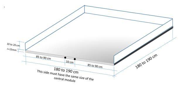
This module should contain holes that allow fitting walls of 10cm to 20cm to the platform. These inner walls have a size of approximately 90cm, with the same thickness of the wall of the module. They are white MDF with two holes for pins, as below:
