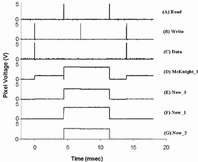
Fig. 9. Measured voltage levels of input signals and four frame buffer pixel capacitors.
