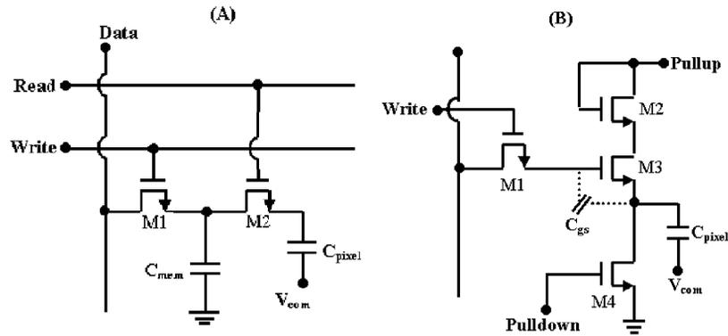
Fig. 3. Frame buffer pixel circuits. a) Proposed by Shields. b) Proposed by McKnight.
