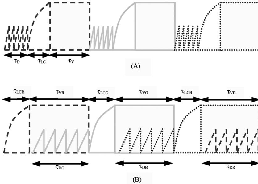
Fig. 2. Illustrations of (a) line-at-a-time driving scheme and (b) frame-at-a-time driving scheme.
