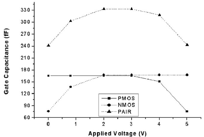
Fig. 6. Voltage-dependent gate capacitance of PMOS and NMOS. Width and length are 7.5 and 9.5  $\mu\text{m}$ , respectively.
