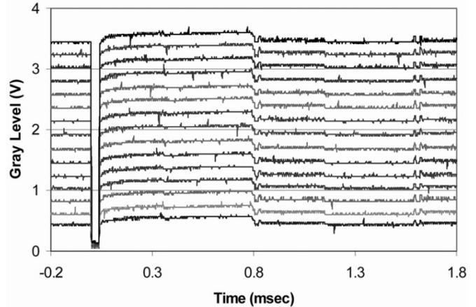
Fig. 10. Fifteen levels of voltage at the pixel electrode formed according to data voltage.
