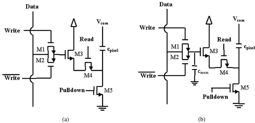
Fig. 5. New frame buffer pixel circuits: (a) with intrinsic gate capacitor and (b) with separate capacitor.
