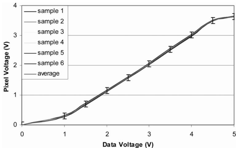
Fig. 8. Voltage on the pixel electrodes with respect to the data voltage.
