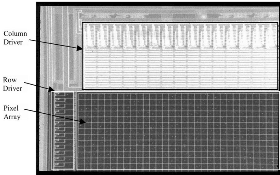
Fig. 7. Left upper corner of the fabricated  $64 \times 32$  microdisplay with frame buffer pixels.
