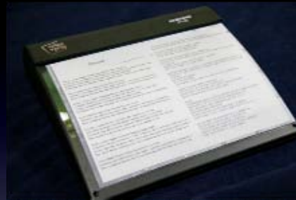
Samsung a-Si on plastic, 130 C process A4 EPD
