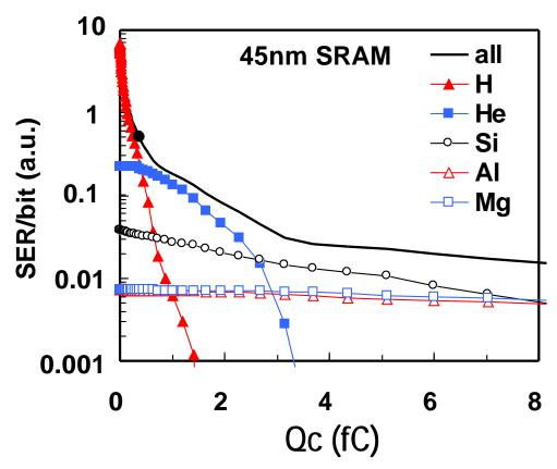
The sharp rise below 0.6fC (13.5keV) is due to the direct ionization of protons
