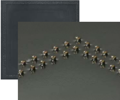
Top view of overmolded bottom package
