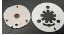
LED array board (shown without LUXEON LEDs and thermal interface material) LED white reflector sheet
