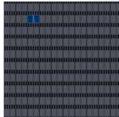
Figure 6. Resistor and Bump locations 10x10 array, 1mm unit cell
