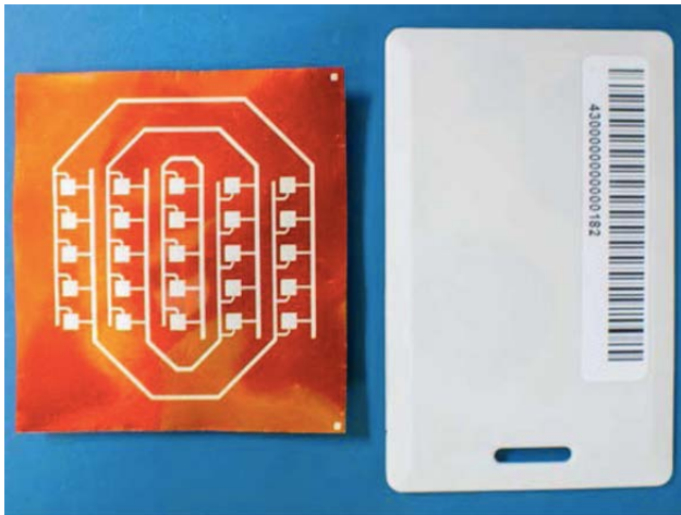
25-Patch Van-Atta reflect array printed on Kapton. The area similar to a credit card or traditional RFID card
