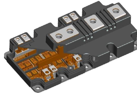
For copper bonding a copper chip metallization is needed
