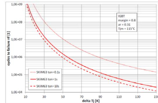
Lifetime Models for a certain IGBT module technology showing the impact of power cycle **ton** times at a given **aspect ratio** of the bond loop
