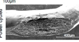
Fine microstructure (~1 µm) at the bonding interface
