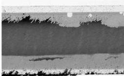
"Corroded Electrodes" 10mm
