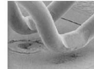
Investigating the thermo-mechanical fatigue of 400 $\mu$ m Al bond wire interconnects with respect to bond wire lift-off failure
