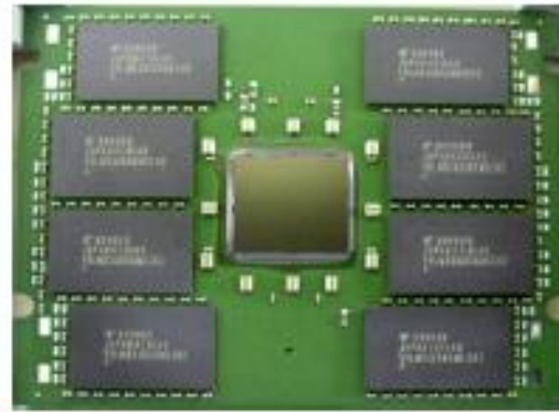
55 x 72 mm, Network Switch, ASIC + Memory
