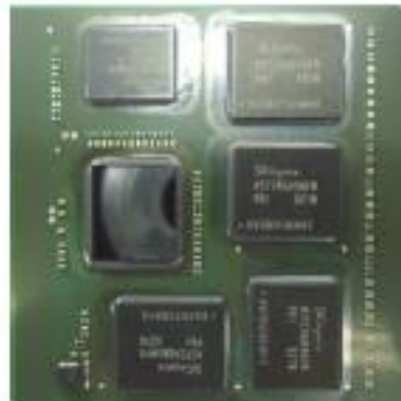
42.5 x 42.5 mm, Infotainment, Processor + DDR
