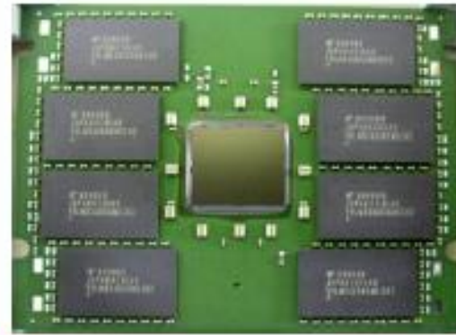
55 x 72 mm, Network Switch, ASIC + Memory
