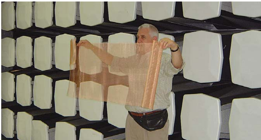
Colin Brench of HP holds up a copper screen which was used to demonstrate how the technique easily picked up that irregularity in the semi anechoic ten meter chamber which was made available to the ANSI ASC C63 committee by Northwest EMC.
