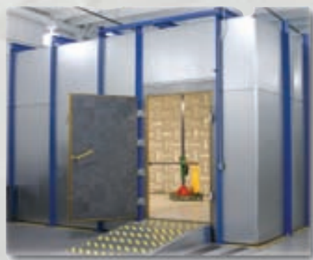
3 Meter EMC Chamber
