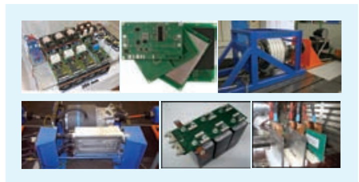
Figure 2. Research activities at ISEA (from top-left): Highly efficient PV converter, PCB-integrated active and passive components, 120 kW railway-drive test bench, 100 kW, 15,000 rpm automotive-drive test bench, charge balancing circuit for batteries, characterization of Li-Ion battery cells in thermal chamber
