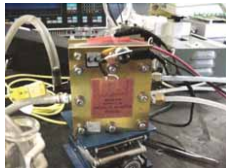
Fig. 6 DMFC experimental setup
