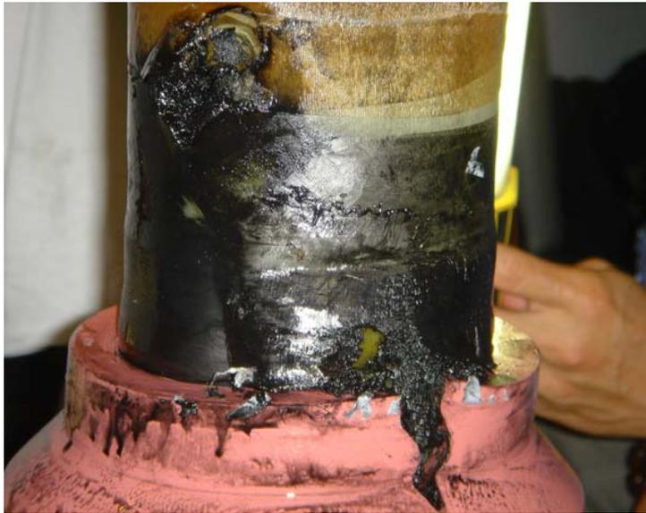
Fig. 4: Cable breakdown
