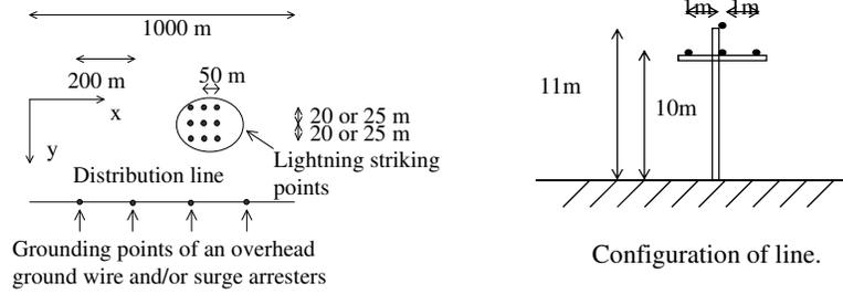
Fig.1. Arrangement of distribution line and lightning striking points.
