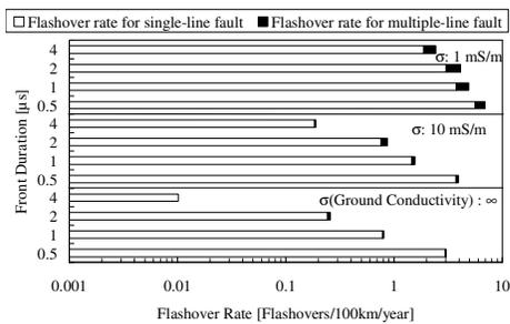
Fig. 6. Flashover rate of the line equipped with a ground wire calculated without taking account of the correlation between the peak values and the front duration of the return-stroke current waveform.
