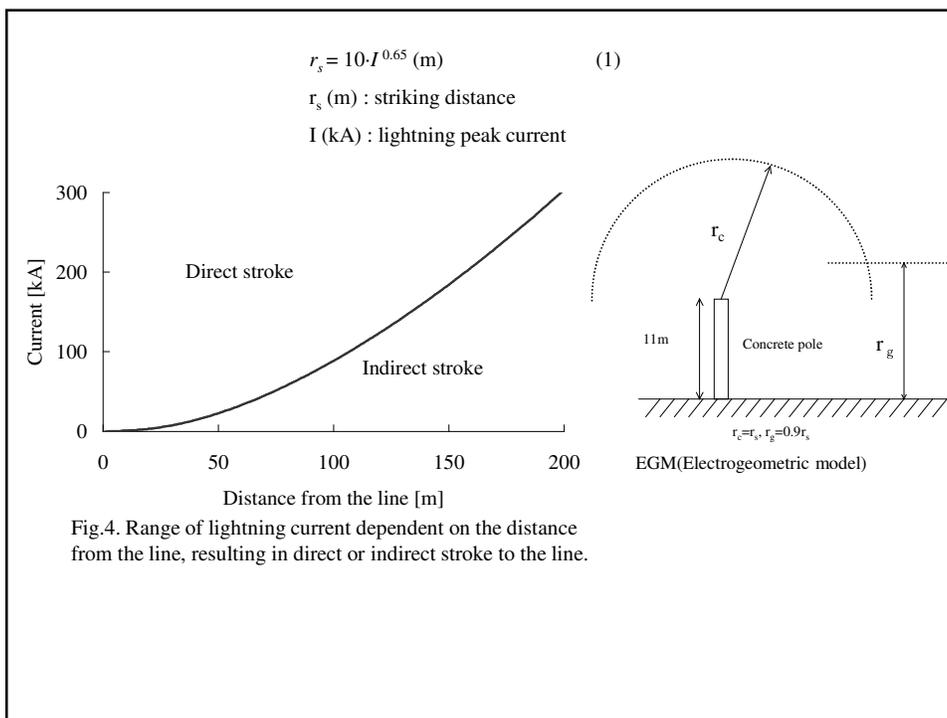
Fig.4. Range of lightning current dependent on the distance from the line, resulting in direct or indirect stroke to the line.
