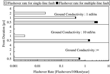
Fig. 5. Flashover rate of the line equipped with surge arresters calculated without taking account of the correlation between the peak values and the front duration of the return-stroke current waveform
