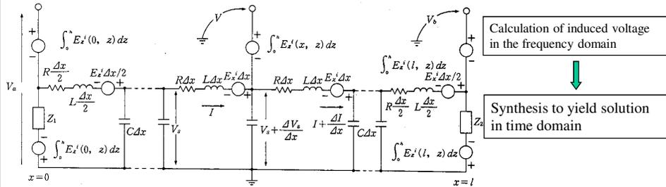
Equivalent circuit of an overhead wire for calculation of induced voltage :
