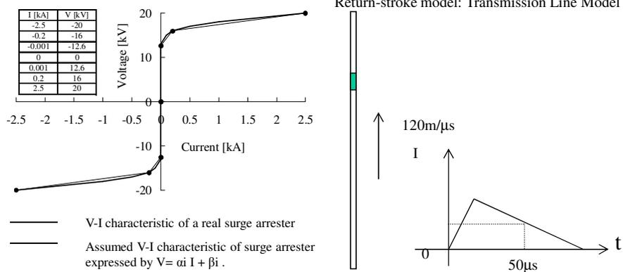
Fig.2. Assumed V-I characteristic of surge arrester passing points in the table.
