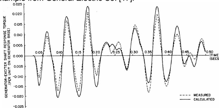
Shaft Torque Comparison of Calculated Results to Actual
