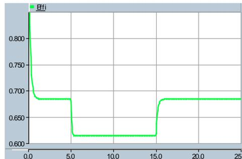
Figure 4. PEMFC output efficiency.
