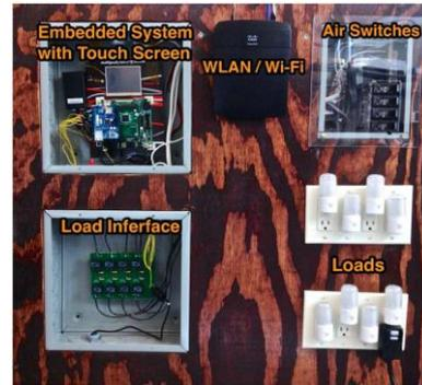
Fig. 3 Prototype platform of SHEMS
