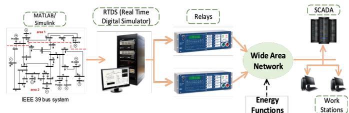
Fig. 2. Integrated setup for real-time testing of the proposed approach on blackout sequence
