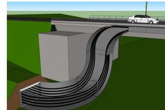
Fig. 3. Schematic illustration of the transition from the tunnel to the bridge.
