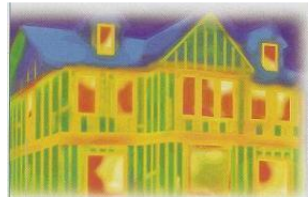
Cavity Insulation with OSB Sheathing
