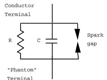
The principal characteristic of an insulator is that, normally, the values of resistance, capacitance, and spark-gap breakdown voltage are sufficiently high (low for the capacitance element) that they can be ignored as circuit elements.
