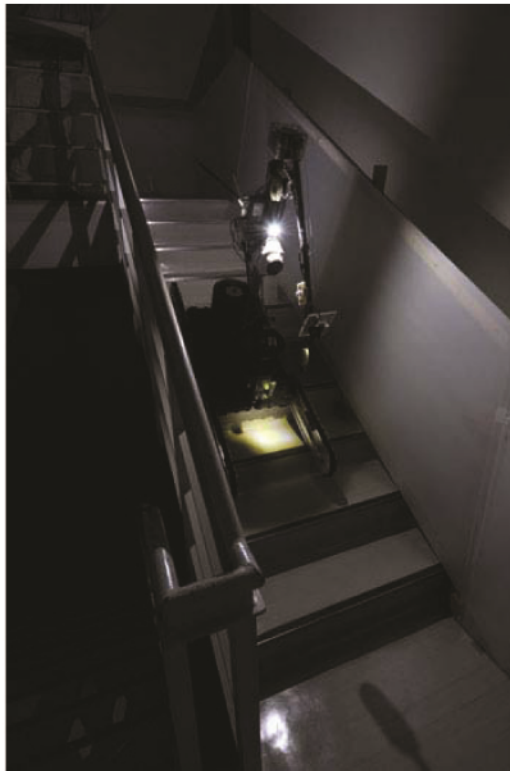
Slinky move: Quince moves down stairs at Chiba Institute of Technology by IURA, CHIBA INSTITUTE OF TECHNOLOGY
