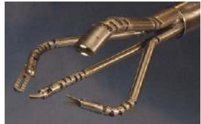
Research SILS robot: Intuitive Surgical prototype for single port surgery
