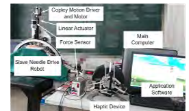
Experimental setup of needle driving force feedback
