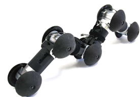
The Proposed In-pipe Robot with Underactuated Twisting Joints
