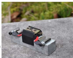
Device for In-Situ Measurement of Concrete Corrosion
