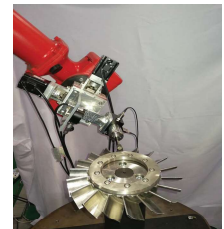
Robotic Compliant Grinding for Complex Blisk
