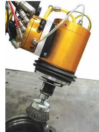
VersaFinish ACT-390 Axially-Compliant Finishing Tool
