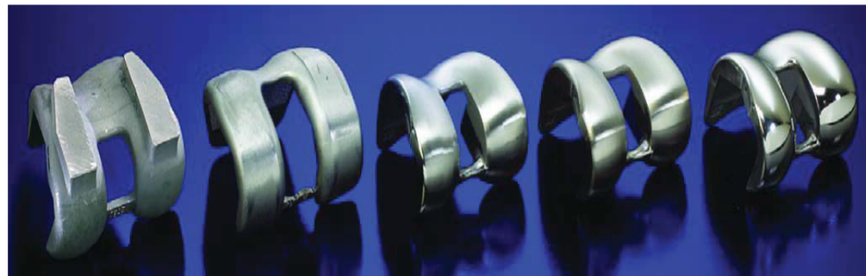
Gate removal grinding
