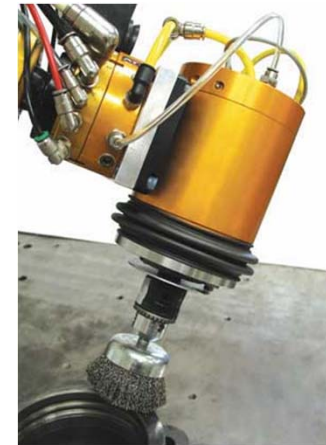
VersaFinish ACT-390 Axially-Compliant Finishing Tool
