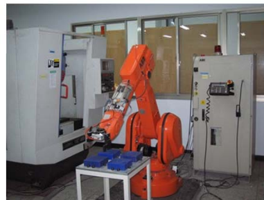
Robot loading/unloading machining system
