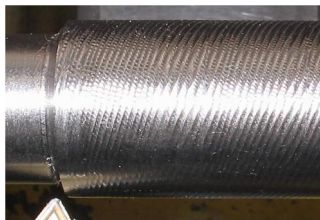
texture caused by chatter in turning
