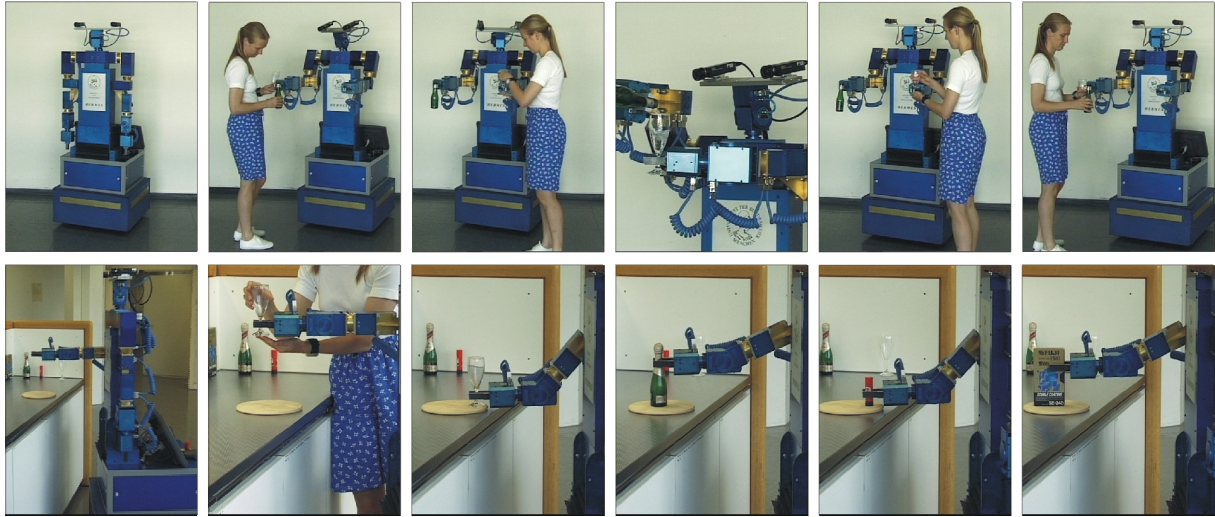
Fig. 7. Motion sequences for demonstrating tactile sensing skills; top row: interacting with a human and filling a glass with water (from left to right: robot standing by, taking over bottle from a human, taking over glass, visually supervising filling action, handing over glass to a human, handing over bottle); bottom row: taking over various objects from a human (glass, bottle, glue stick, video cassette) and placing them gently onto a tray
