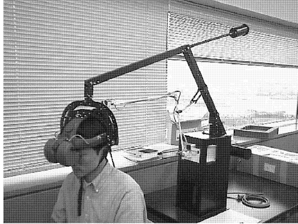
Fig. 7. Developed HMD system with head-tracking
